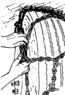
Tighten with the tightening cam by inserting a tightening lever into the groove of the cam and twisting it 90 degrees so that the chain loop slips into the locked position (6).
