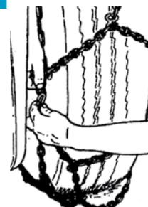
**4** Then tighten the chain around the wheel manually by pulling the outer side chains together. Then hook the outer side chains together.
