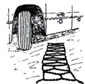
**2** Lift the chain onto the wheel with the tightening cams on the outside and in a "slack" position. Push the end of the chain in under the back of the wheel and reverse the vehicle by about 1/4 turn of the wheel.
